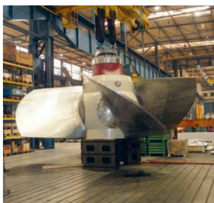
□ Kaplan runner during manufacturing
